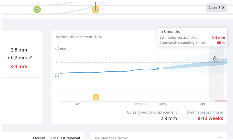
Figure 2.7: The figure shows a screenshot of the KONUX Switch product. In more detail, one sees a graph showing the vertical displacement in the past and predicted for the future. In addition, percentage value for exceeding the critical 3mm is given for future values. [2]
