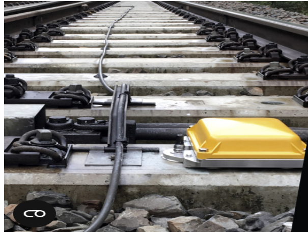
Figure 2.3: The figure shows the final form of the KONUX Switch sensor, installed within the trackbeds. The external yellow protective casing is also visible, which further protects the sensors from any damage from outside. [2]
